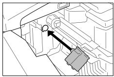
9 Align the grid cleaner with the notch and attach it to the machine.
